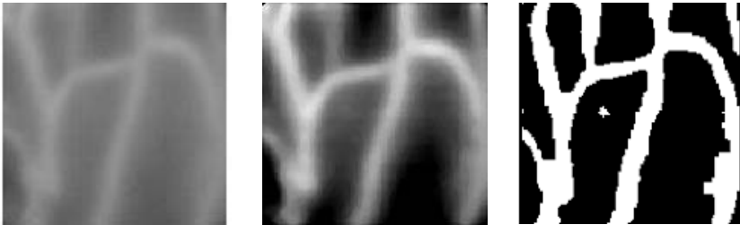
Fig. 4. Left: Region of interest; Center: After normalization; Right: After local thresholding.
