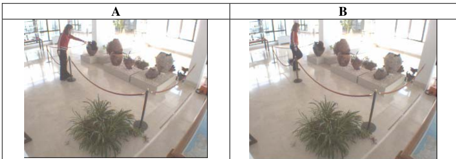
Fig. 3. Two critical situations: A) a visitor stays behind the limit of the forbidden area but he seems very close to the find due to the perspective projection onto the image plan; the proposed system avoid the error of the perspective perception and classifies as normal this behaviors. B) A visitor is inside the limit of the forbidden area. In this case the position estimation indicates the access violation and an alarm can be provided.
