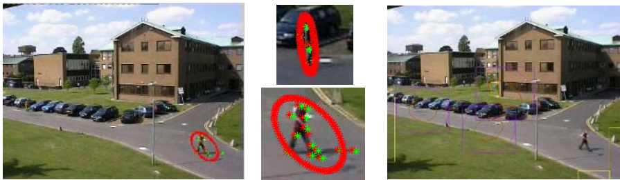
Fig. 7. Comparison of the method with our previous work which integrates background subtraction and motion history detection in the framework of a Kalman filter [14]. As expected, the track of the pedestrian is lost during the rapid illumination changes, shown in the right panel, whereas our new method succeeds in tracking in such situations, shown in the left panel. In the middle panel, two subimages of the same pedestrian at different time are displayed to show how the parameters of the cluster are affected by the shadow.
