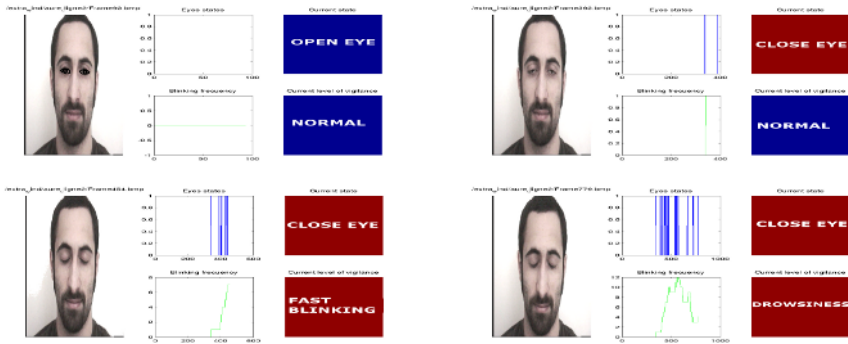
Fig. 10. Estimation of the vigilance. For each figure: left: current image; middle, top: past evolution of the eyes states, bottom: past evolution of the blinking frequency; right, top: current detected eye state, bottom: current vigilance level.
