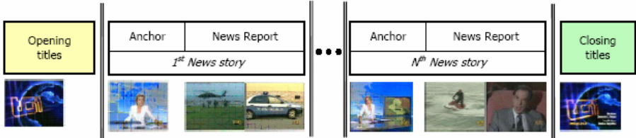
Fig. 1. The typical structure of a news video: the opening titles , a sequence of N news stories and the closing titles .
