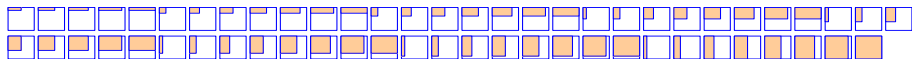
Fig. 1. Example spatial templates with the top left point (0, 0) for 64 \times 64 image. The orange rectangles are the masks used to calculate histogram feature.
